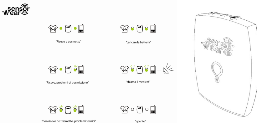
Fig. 2. The ergonomic study for the user interface and the device shape as regards wearability issues.
